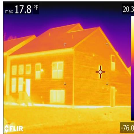
With Exterior Continuous Insulation
